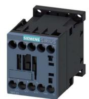
power contactor, AC-3e/AC-3, 9 A, 4 kW / 400 V, 3-pole, 230 V AC, 50/60 Hz, auxiliary contacts: 1 NO, screw terminal, size: S00
